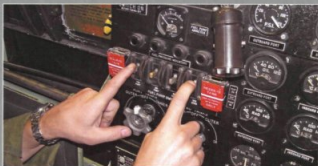
14 The outer tank fuel pump is set to ON
