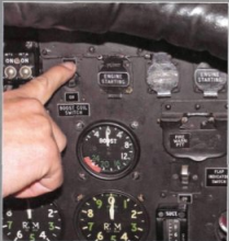
5 The boost coil switch is set to ON
