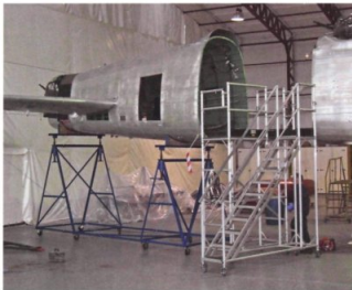
ABOVE The aircraft is jacked and trestled. All the engines, engine bearer frames and undercarriage legs have been removed. (Bruce Irvine)
