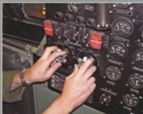
13 The fuel tank selector cocks are moved to the OUTER TANK position
