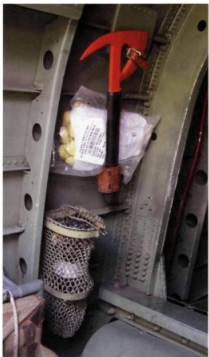
FAR LEFT First-aid outfit, stowed on the starboard side aft of the entrance door and accessed by pulling the handle. (Jarrod Cotter)
