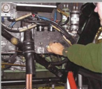
17 He then operates the pump 8 to 12 times to prime the engine
