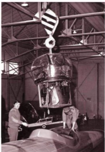
LEFT A major milestone in PA474's restoration to authentic wartime configuration was the fitting of a mid-upper turret, seen here being lowered into position during 1976 under the guidance of Pete 'Gerbs' Jeffery and Engineering Officer Flight Lieutenant Terry Lees. (Crown Copyright)
