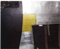
RIGHT Skin repair work to the underside of a wing. (Crown Copyright)
