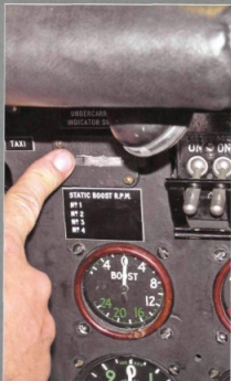
3 The undercarriage master switch is set to ON
