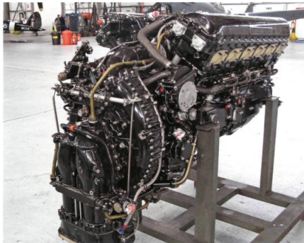
LEFT Merlin 25 viewed from the rear, showing the supercharger unit and carburettor clearly. (Paul Blackah/Crown Copyright)
