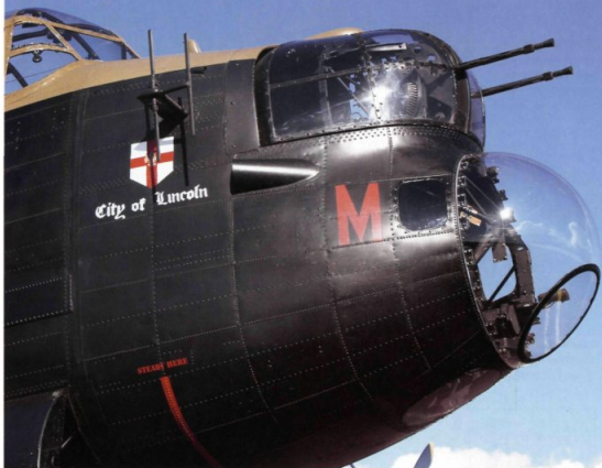
ABOVE PA474's nose, with the FN5 front gun turret prominent. (Jarrod Cotter)
