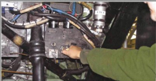
16 The person in the undercarriage bay unscrews the priming pump
