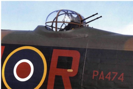
ABOVE PA474's nose, with the FN5 front gun turret prominent. (Jarrod Cotter)
