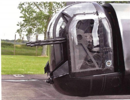
LEFT External view of the FN121 rear turret, fitted with four Browning 0.30in machine guns. (Paul Blackah /Crown Copyright)
