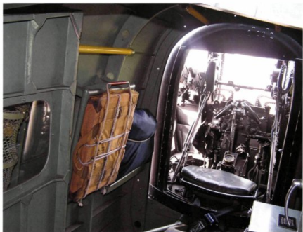
LEFT Entrance to the rear gun turret, showing the gunner's parachute stowage position. (Paul Blackah/ Crown Copyright)
