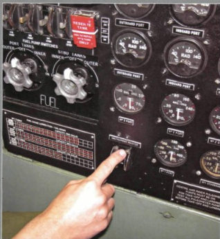
4 At the same time the instrument panel switch is set to ON
