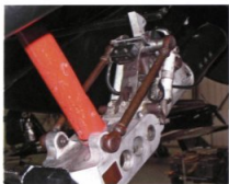
TOP The non-retractable tailwheel. (Paul Blackah/Crown Copyright)
