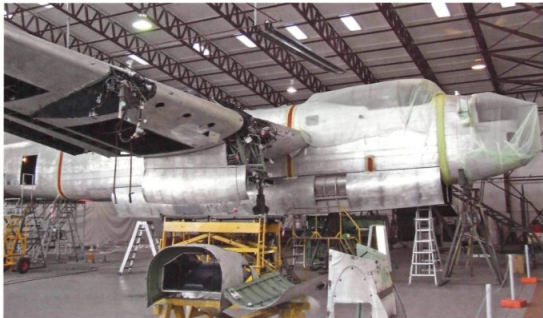
ABOVE The aircraft is jacked and trestled. All the engines, engine bearer frames and undercarriage legs have been removed. (Bruce Irvine)
