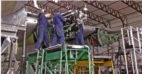
ABOVE Engine refit in progress. (Bruce Irvine)
