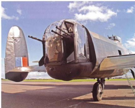
LEFT General view of the tail unit, with the elevators seen in the lowered position that would cause the aircraft to adopt a nose-down attitude in flight. (Jarrod Cotter)
