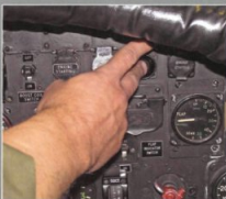
18 The switch guard is lifted, the number 3 engine start button is pressed and the engine starts
