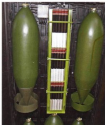
FAR RIGHT A mix of 1,000lb and 500lb High Explosive GP bombs and an incendiary container in the bomb bay of a Lancaster. (Jarrod Cotter)
