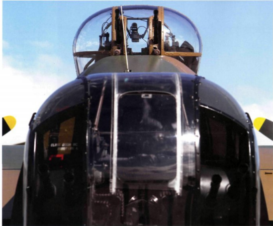
ABOVE Six of the eight Browning 0.303in machine-guns installed in PA474's turrets pointing rearwards. (Jarrod Cotter)
